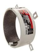
B1 Fire Collar is designed to maintain the fire resistance of fire rated walls and floors where these are breached by continuous plastic pipes, and may be used in gypsum, masonry and concrete walls and floors. The steel shell contains a graphite based reactive material which reacts when exposed to heat closing the openings left by the softening plastic pipe in fire.
